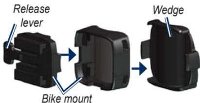
**For horizontal bars:** Separate and remove the top part of the mount, turn it 90 degrees, and replace it. Continue with step 2.
