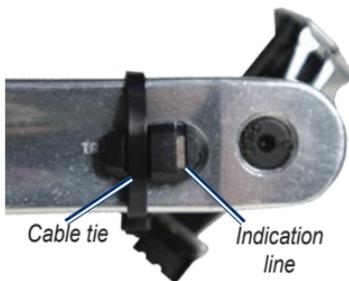
**Pedal magnet on crank arm**
