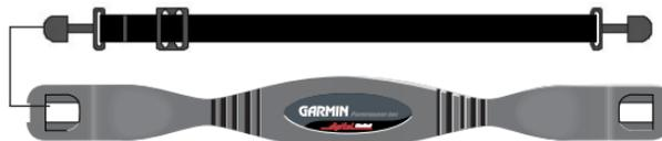
2. Wet both sensors on the back of the heart rate monitor to create a strong connection between your pulse and the transmitter.
