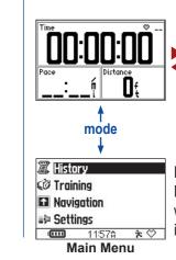
Press mode to view the Main Menu. Using the Main Menu, you can set up simple or advanced workouts, view your history data, save locations in memory, and customize the Forerunner.
