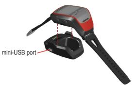
Plug the small end of the AC adapter into the mini-USB port on the cradle. Plug the other end into a standard wall outlet.
