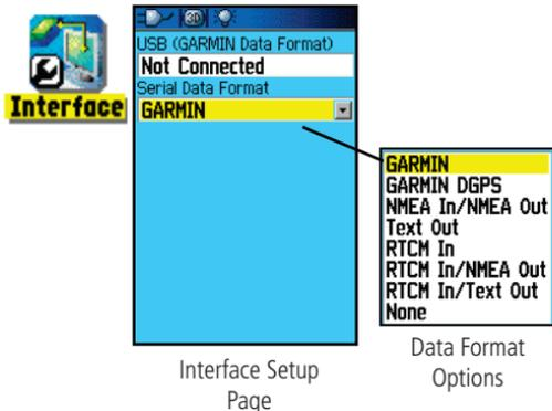
The screenshot shows the 'Interface Setup' menu with the following options: USB (GARMIN Data Format) (Not Connected) and Serial Data Format (GARMIN). Callouts include: 'Interface' icon, 'Data Format Options' list (GARMIN, GARMIN DGPS, NMEA In/NMEA Out, Text Out, RTCM In, RTCM In/NMEA Out, RTCM In/Text Out, None), and 'Data Format Options' label.
