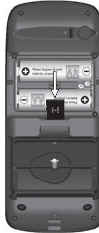
The GPSMAP 76CSx requires two AA batteries (not included), which are located in the back of the unit under the D-Ring. Alkaline or NiMH batteries can be used (see the *Owner's Manual* for setting the battery type). Stored data is not lost when batteries are removed. Install the batteries, observing the proper polarity. A polarity diagram can be found molded into the battery compartment. Extensive use of backlighting, WAAS, and key beep tones can significantly reduce battery life.
