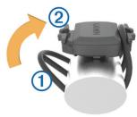
4 Rotate the crank arm to check for clearance.
