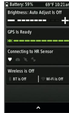
The connections page appears. A flashing icon means the device is searching. You can select any icon to change the settings.
