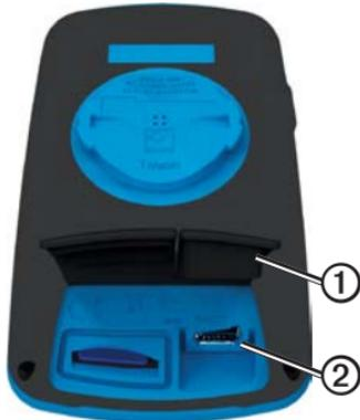
3. Plug the small end of the AC charger into the mini-USB port.
