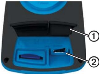
3. Plug the small end of the USB cable into the mini-USB port.
