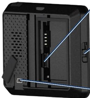
*microSD card slot under the battery*
