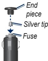
3. Ensure that the silver tip is placed in the black end piece. Screw on the black end piece.
