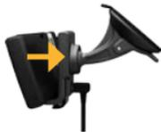
8. Plug the other end of the vehicle power cable into a power outlet in your vehicle.
