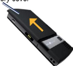
2. Insert the SIM card in the slot at the top of the battery compartment. Insert the notched corner of the SIM card first with the gold contacts facing up. The SIM card clicks into place.
