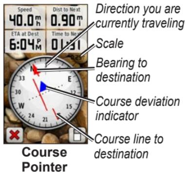
The course pointer provides an indication of drift (right or left)
