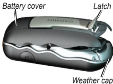
2. Insert the batteries, observing polarity.
