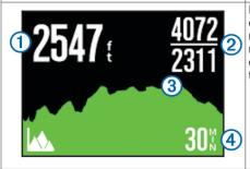
Elevation displays the current elevation ①, maximum and minimum elevations ②, elevation graph ③, and time scale ④.
