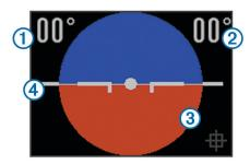
**2** Adjust the device until the degree of roll ① and degree of pitch ② are both 00°, and the brown section of the level ③ is even with the horizon line ④.
