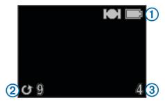
The device takes repeated photos at the selected interval. The viewfinder displays the GPS and battery status ①, the time in seconds until the next photo is taken ②, and the number of repeated photos the device has taken ③.
