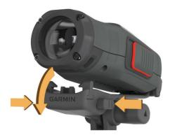
The camera should be held tightly and should not move in the mount when properly secured.
