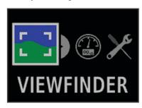
The modes cycle from left to right. The icon for the selected mode appears larger, and the name of the selected mode appears at the bottom of the screen.
