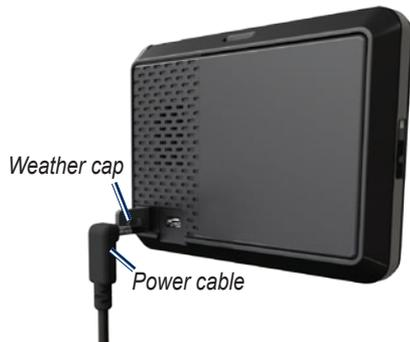
2. Plug the vehicle power cable into the mini-USB connector.
